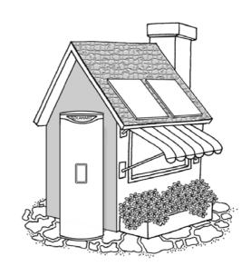
It is recommended the solar storage tank be installed at ground or floor level and must stand vertically upright. Remember all local authorities have regulations about putting water heaters into roof spaces.
